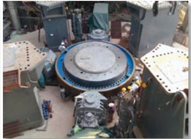
Figure 8: Mounted supports and girth gear of MVR 5600 C-4 at Balaji
