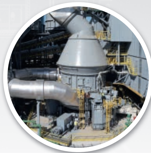
Grinding of cement and granulated blast-furnace slag with MVR vertical mills
