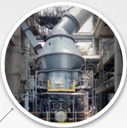
Coal grinding with MPS vertical mills
