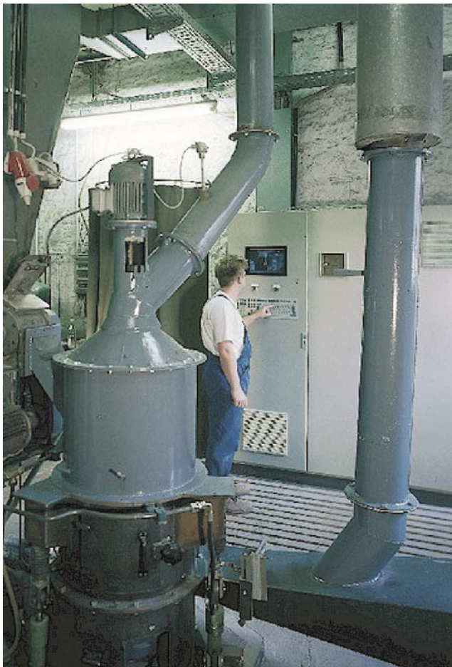
Figure 2: Test plant with an MPS 40B vertical roller mill at the research centre of Gebr. Pfeiffer A.G. in Kaiserslautern
